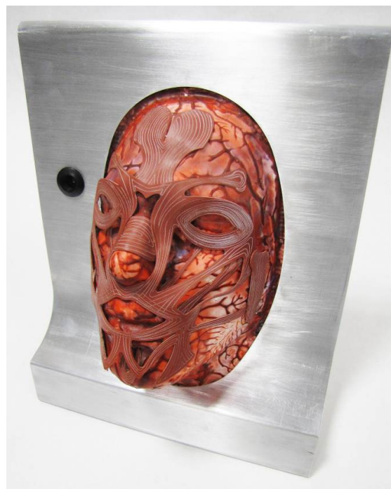
Figure 3 Animatronic model with silicone musculature
